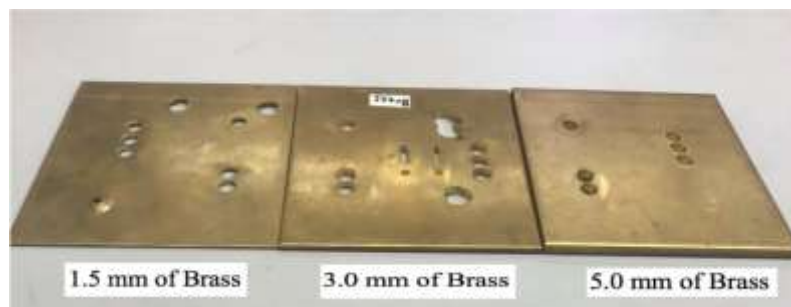
Figure 3.1 The artificial defect on metal (i.e. Brass) with different kind of thickness.
